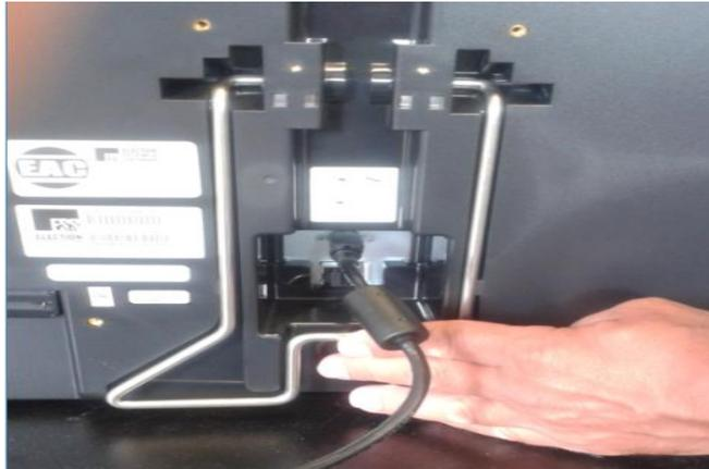
8. Remove the power cord from the back of the ballot marking device by sliding the sheath on the plug back while gently pulling the plug out.
