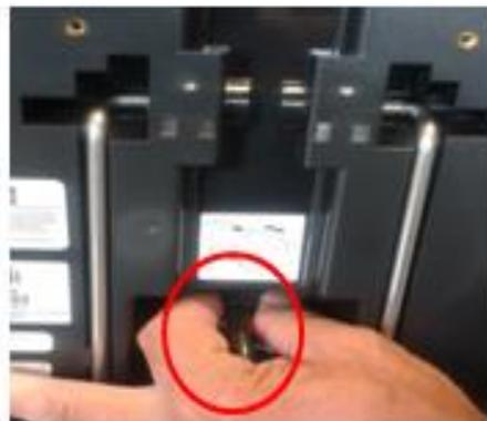
5. Grasp the bottom of the stand on the back of the ballot marking device. Pull out and extend the stand. Rest the ballot marking device on the stand. Position the ballot marking device on the designated table.
