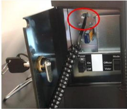
12. Flip the “**Power**” switch to the “**On**” position.
